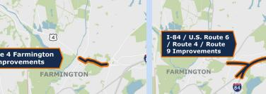
Eliminate left-hand ramps, improve lane balance, and provide movements between Route 4 and Route 9 on the I-84 Interchanges in Farmington.
