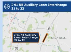
Reduce crash rates and improve traffic operations on I-91 by adding an auxiliary lane between the Route 372 on-ramp and the Route 9 off-ramp.
